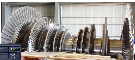
GE 230 MW Turbogas Turbine with GE G60 protection
