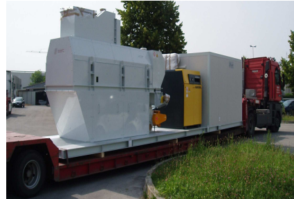
Skid platform for RDF Plant
