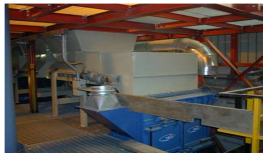
SAET DPN-Speciale series Weight Belt Feeder for CdR and Pfu
