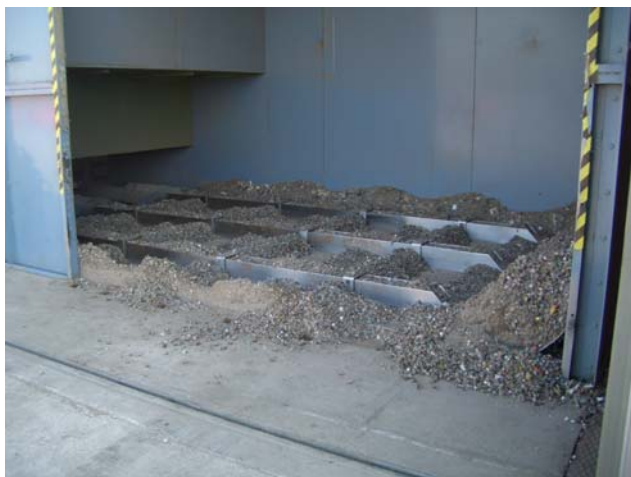
Photo of hopper with moving platform (CdR Receptioning zone)
