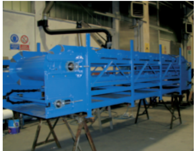
Fig. 3 - The conveyor apron feeder
