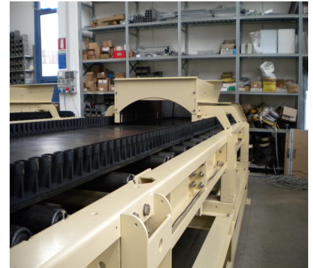
Belt Weigh Feeder in workshop
