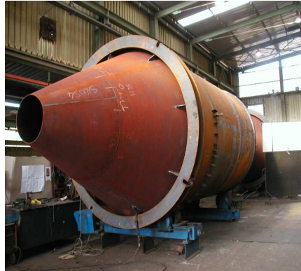
Storage silo in workshop
